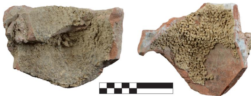
Fig. 8. Calcareous deposits on terracotta water pipes of Parion (Parion arch.)
